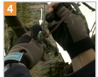
4 Create loop by putting tail through Gripple Plus tensioner
